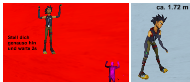
Figure 3.3.: Calibration in KinectWalker . On the left: a virtual avatar of the Unity3D game engine shows how to perform the PSI calibration pose. On the right: the body height is displayed after the calibration process has been finished.
