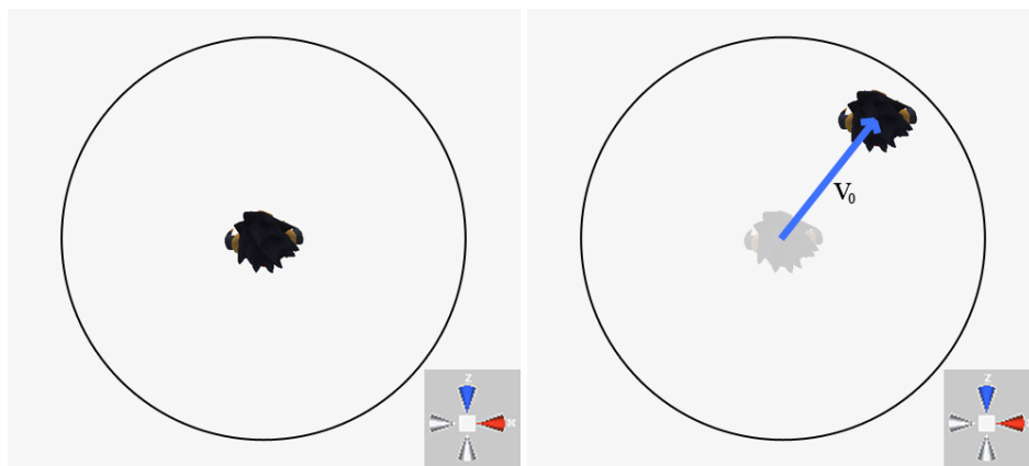
Figure 4.11.: Distance-To-Velocity gesture. On the left: the initial position of the user. On the right: the user has moved and the vector v_0 describes the direction and speed.
