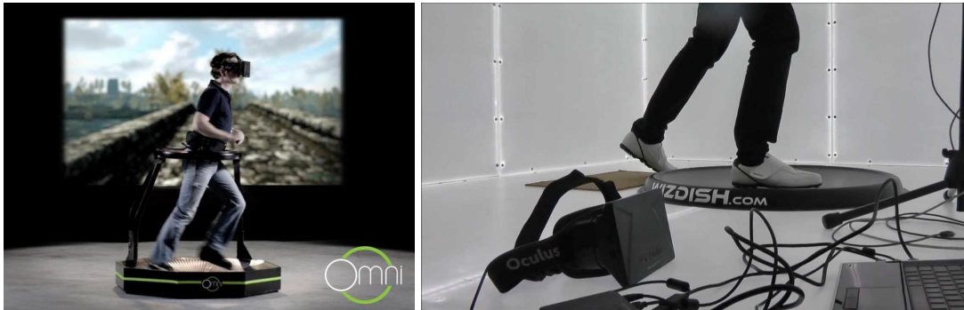
Figure 2.2.: Examples of omnidirectional treadmills. On the left: Virtuix Omni (kickstarter.com). On the right: the Wizdish input device (wizdish.com).
